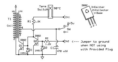
NOTE: Therm Switch heat sink glued to Q1 - both Circuits
